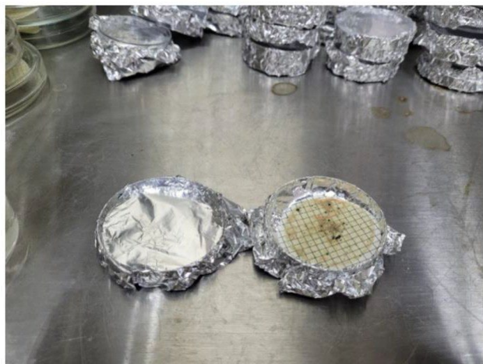
Figure 3. Reduced surface seawater samples on filters for small microplastics collected in the Kuala Terengganu estuary.
