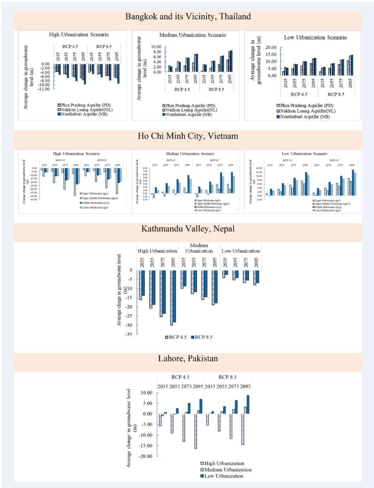
FIGURE 7. The average change in groundwater level for both RCP scenarios (RCP 4.5, RCP 8.5), three land-use change and pumping scenarios (low, medium, and high urbanisation) for four future periods: 2035, 2055, 2075 and 2095 relative to the baseline in four Asian cities.
